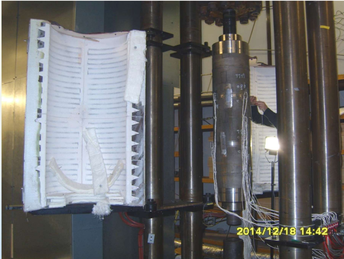
P91 pipe with two butt welds being tested at temperature, under pressure and end load to simulate system loads
